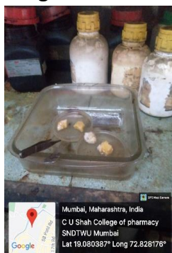
Storage of sodium immersed in kerosene
